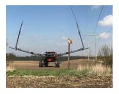
If equipment comes into contact with a power line, assume the line is energized and deadly. The operator should NOT get off the machinery unless in immediate danger. If the operator touches the ground and the equipment at the same time, they will become a channel for electricity. Instead, the operator should stay on the equipment and contact the local electric utility or 911 immediately to report the incident so power lines can be deenergized safely before exiting.
